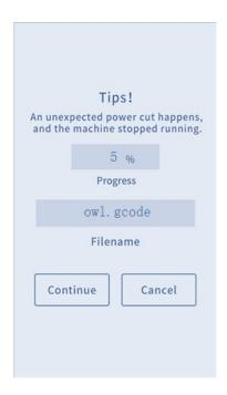
Tips: Before resuming, please clean the excessive filament on the nozzle and model to avoid affecting the printing quality.
